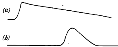
Figure 28. The shape of heat pulses through liquid helium and viewed on an oscilloscope trace: (a) pure ^4\text{He} at 0.45^\circ\text{K} , (b) ^4\text{He} containing 0.32\% ^3\text{He} at 0.45^\circ\text{K} (after King and H. A. Fairbank 1954).
