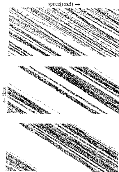
Fig. 47. Typical space-time diagram of the NaSch model with v_{max} = 2 and c = 0.1 and random braking probabilities. Each horizontal row of dots represents the instantaneous positions of the vehicles moving towards right while the successive rows of dots represent the positions of the same vehicles at the successive timesteps.
