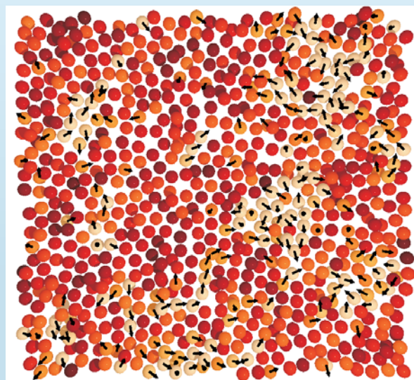
Figure 2. A thin slice through a colloidal gel illustrates the heterogeneous dynamics of component particles. Arrows indicate the direction of motion for particles with displacements greater than 0.2 \mu\text{m} over a time interval of 600 seconds; lighter colors signify particles with larger displacements. The arrows are all the same length in three dimensions, so shortened arrows indicate motion into or out of the plane. (Adapted from ref. 10, E. R. Weeks, D. A. Weitz.)
